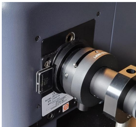
Figure 29: The fixed slit holder at the output port of the monochromator, with slit installed in proper orientation, label facing away from monochromator
