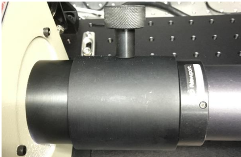
Figure 33: Rear reflector adjustment knobs on the side of the lamp housing.
