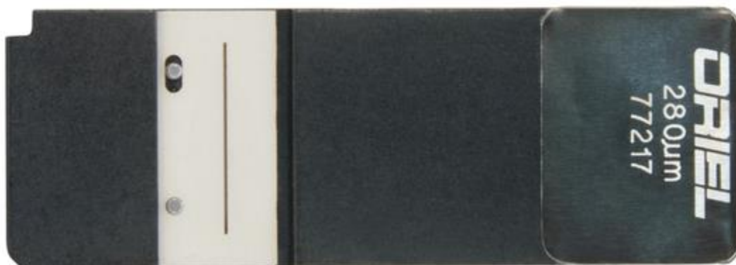
Figure 30: A 280 \mu\text{m} fixed slit with the label oriented outward
