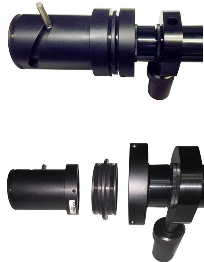
Figure 47: The 77330 Focusing Lens Assembly coupled to the TLS. The bottom view shows the 77792 male-male flange for mechanical coupling.
