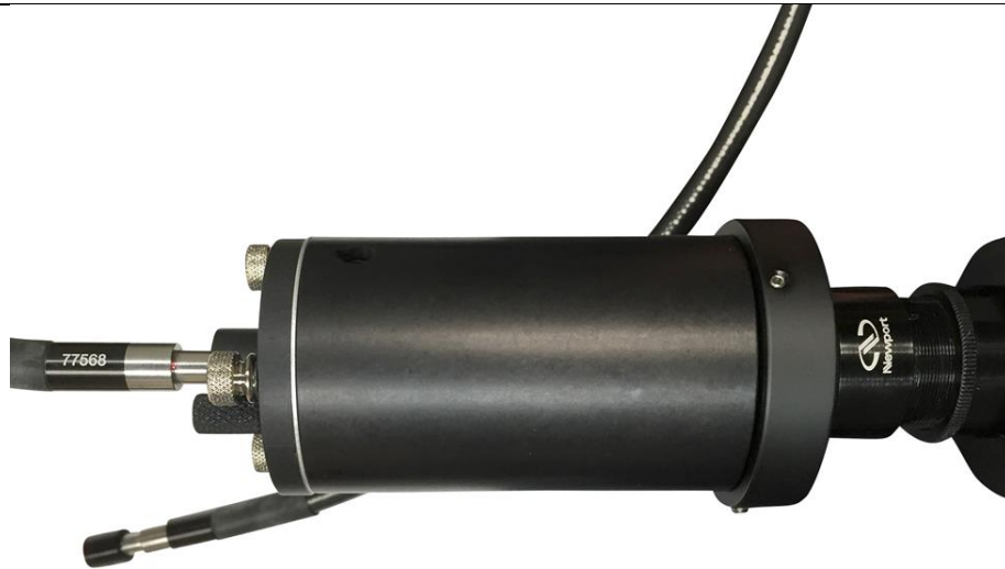
Figure 48: Fiber bundle coupled to the output of the TLS with a fiber bundle focusing assembly.
