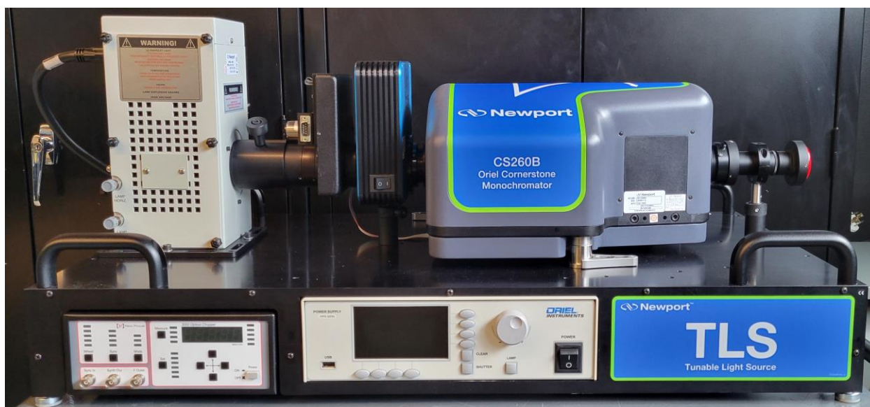
Figure 52: Example of 75160NF chopper system fully integrated in a TLS260B
