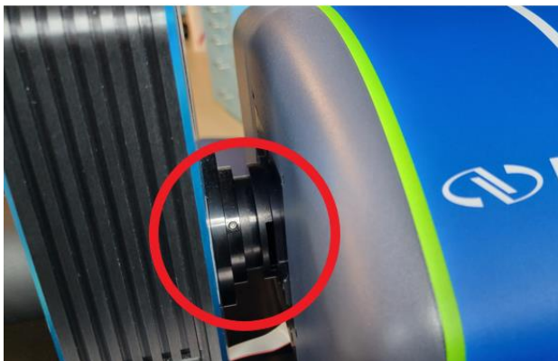
Figure 28: The fixed slit holder at the input port of the monochromator.
