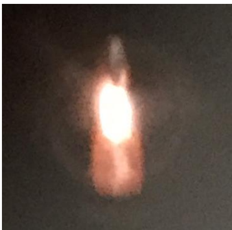
Figure 42: Xe arc lamp output with primary arc image centered.
