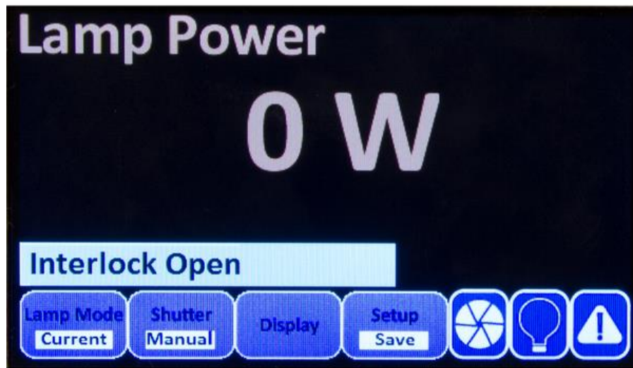
Figure 12: Interlock Open Error Message of the OPS Series Power Supply
